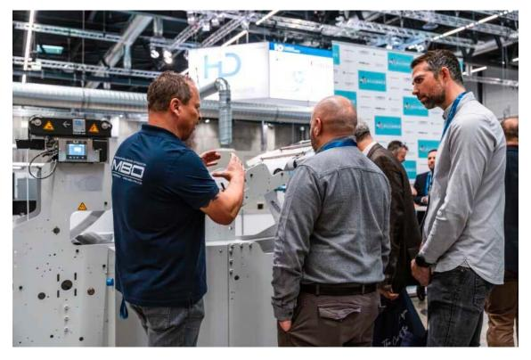
Another key attraction was the Hohner Digifinisher HHS-Futura, showcased in roll-fed mode alongside the MBO UW23 unwinder, SVC525C cross cutter, and folding machine. This setup demonstrated selective finishing capabilities, including variable page numbers and variable cutting thicknesses, essential features for the flexible demands of modern digital print workflows.
