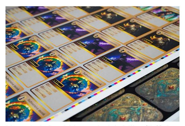
A demonstration of trading card printing was conducted using the Lithrone GX40RP advance EX Edition, which has a five-color front and five-color back configuration. This Lithrone GX40RP advance is equipped for the first time with a coating unit on the RP section, allowing one-pass double-sided varnish coating. The process was managed by the KP-Connect Pro manufacturing execution system, with automatic job data transfer, plate output, and plate transport.
